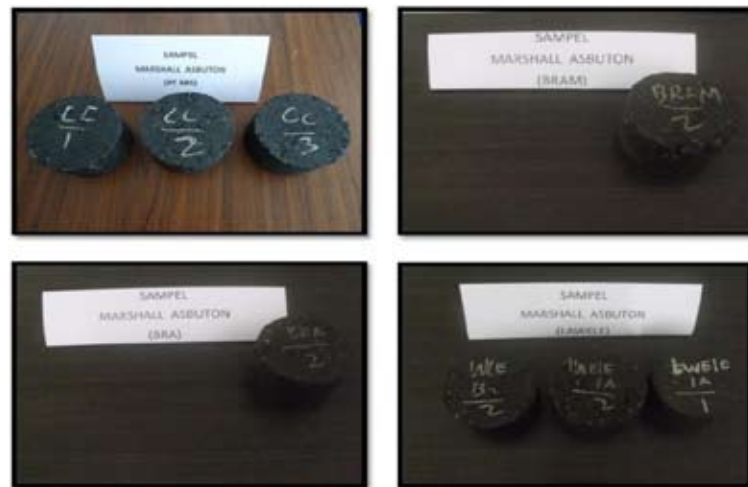
Gambar 3.1-5 Sampel Marshall Asbuton
