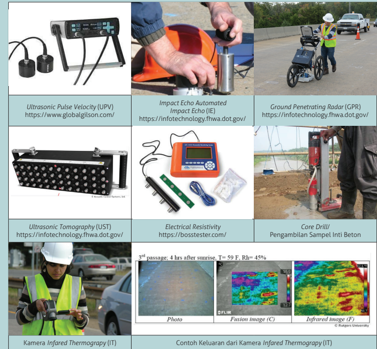
Gambar 13 Penjelasan Gambar Pengujian Ultrasonic Pulse Velocity, Impact Echo, Ground Penetrating Radar, Ultrasonic Tomography, Electrical Resistivity, Core Drill/ Pengambilan Sampel Inti Beton, dan Infrared Thermography
