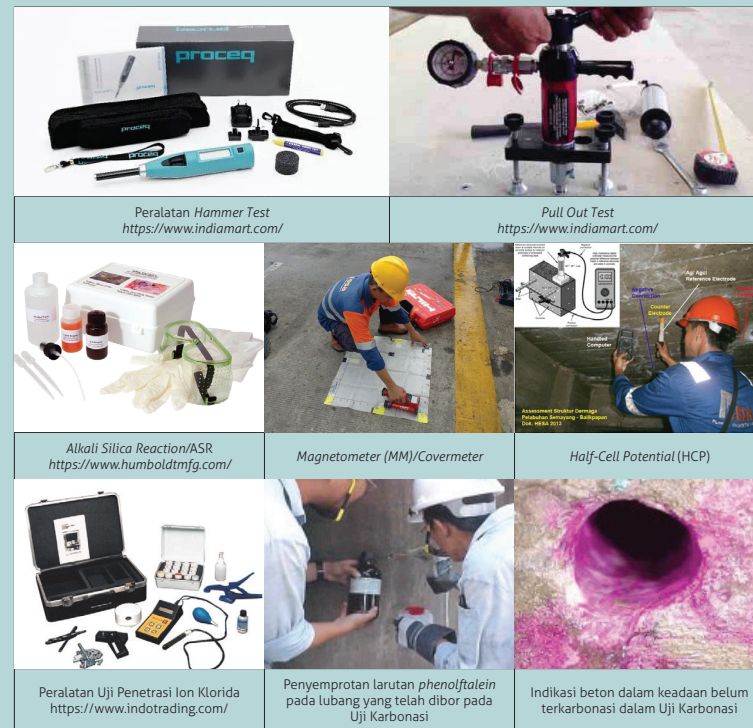
Gambar 14 Penjelasan Gambar Pengujian Pull Out Test, Half-Cell Potential, Hammer Test, Magnetometer, Alkali Silica Reaction, Uji Karbonasi, dan Uji Kadar Klorida
