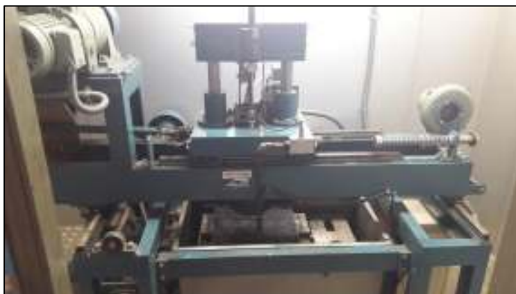
Gambar 3-3. Alat Wheel Tracking Machine (WTM)
