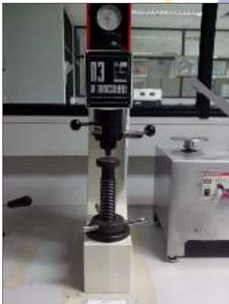
Gambar 12 Alat uji kekerasan (ball indentation)
