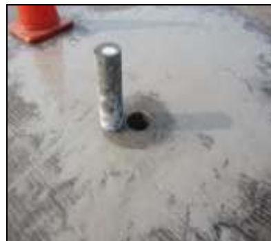
Gambar 6-6 Contoh benda uji hasil core drill
