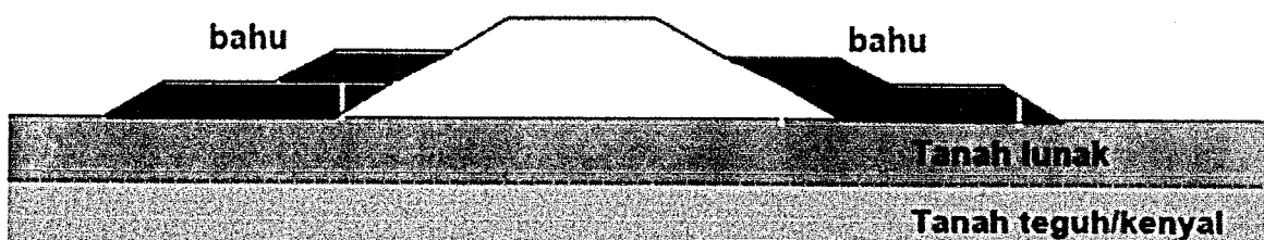
Gambar 2.15 Bahu Beban Kontra Ganda ( Multiple Counterweight Berms )
