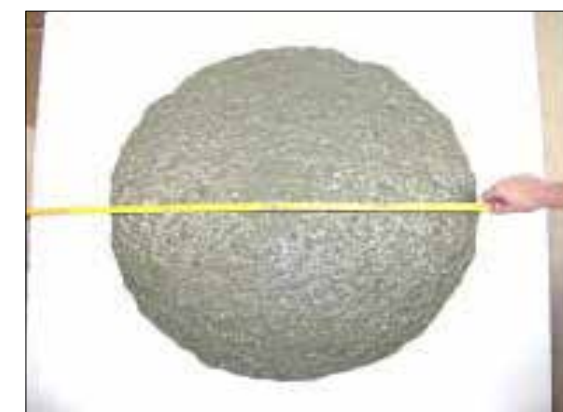
Gambar 9. Pengujian slump flow beton
