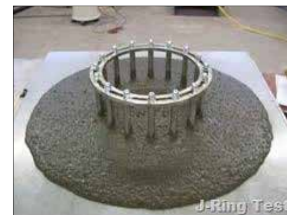
Gambar 10. Pengujian slump flow beton (J Ring Test)
