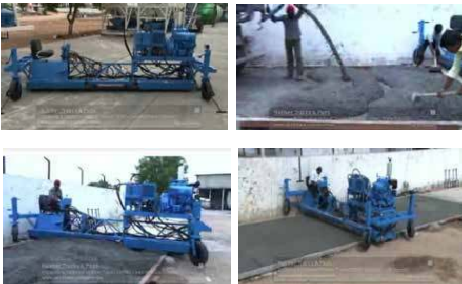
Gambar 17 Apollo Fixed Form Concrete Paver di India ( http://www.youtube.com/watch?v=ms0mcTxMAHo )
