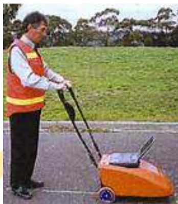
Gambar 99 Alat Walking Profiler
