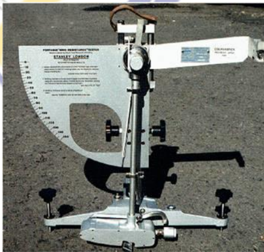
Gambar 3. Alat uji British Pendulum Tester (BPT)
