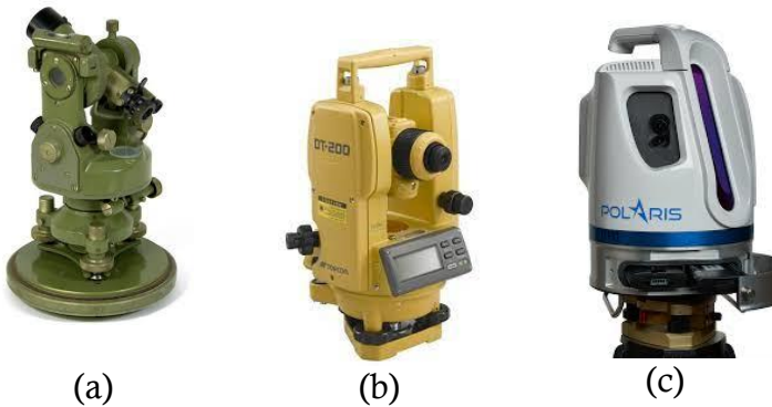
Gambar 73 (a) Theodolite , (b) Electronic Total Station (ETS), (c) Terrestrial Laser Scanning (TLS)
