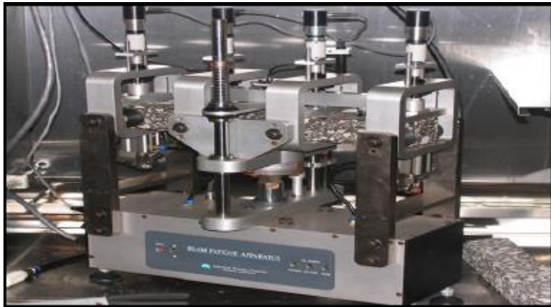
Gambar 5-20. Alat Beam Fatigue Apparatus (BFA) atau Four Point Bending Apparatus
