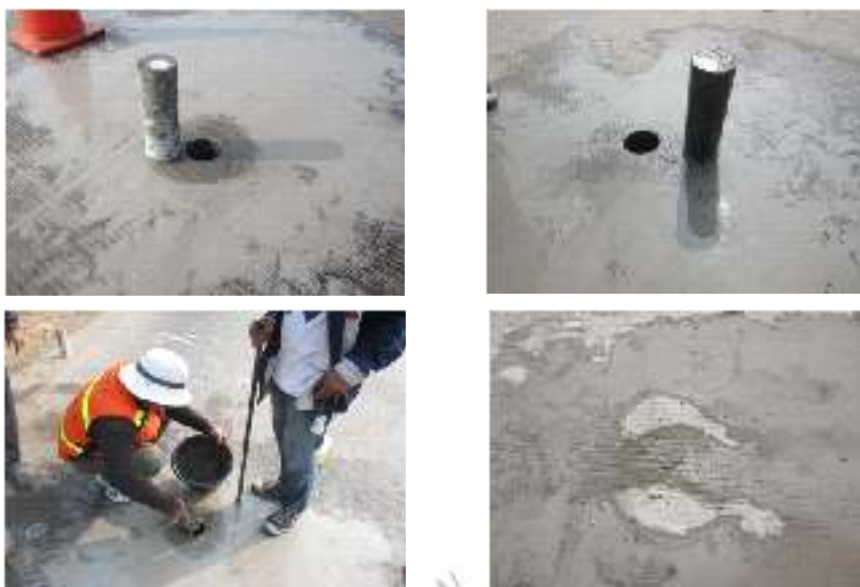
Gambar 4. 13 Pengambilan contoh coredrill
