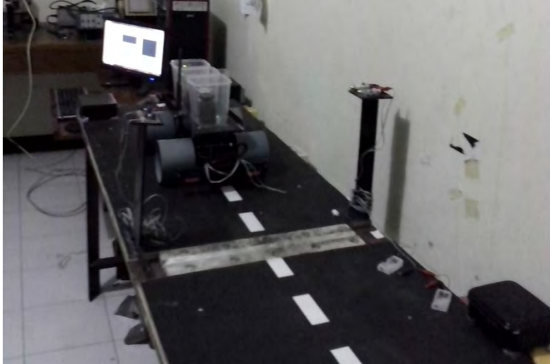
Gambar 22 Set up simulasi weigh in motion
