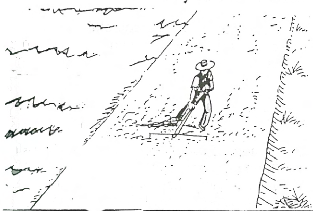
fig. 5. SPREADER RAKE TO SPREAD CEMENT OVER ALL THE SURFACE
