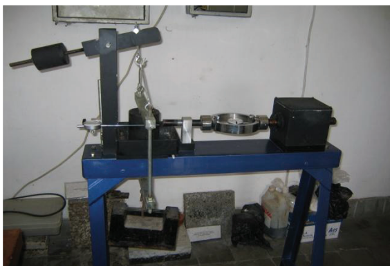
Gambar 6b. Tampak samping alat uji geser
