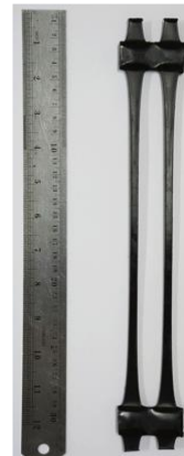
GG4 ( High Density Polyethylene , HDPE Integral Geogrid)
