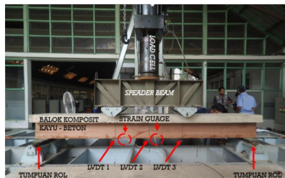
Gambar 2. Set up Balok Uji
