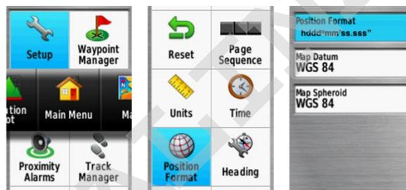
Main Menu -> Setup -> Position Format -> Select "hddd°mm'ss.sss"' - "WGS 84" For Map Datum - "WGS 84" For Map Spheroid -> ENTER/QUIT
