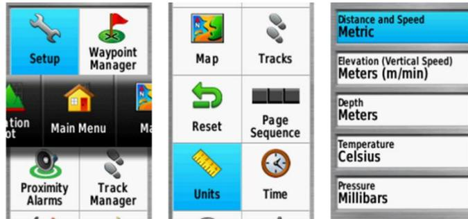
Main Menu -> Setup -> Units -> Select "Metric" For Distance and Speed - "Meters" For Elevation - "Meters" For Depth -> ENTER/QUIT
