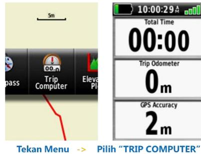
**Gambar 59.** *tracking* – membuka menu Trip Computer
