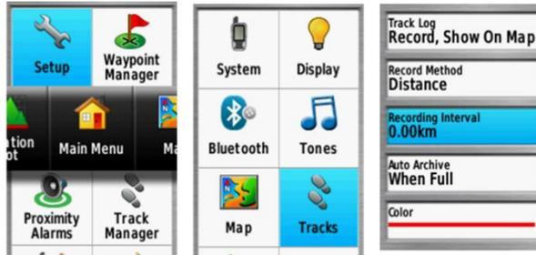
Main Menu -> Setup -> Tracks -> Select "Distance" For Record Method - "0.00km" For Recording Interval -> ENTER/QUIT
