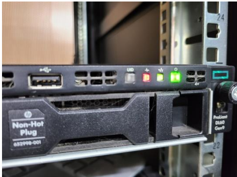
(a) DAQ server health LED yang berkedip
