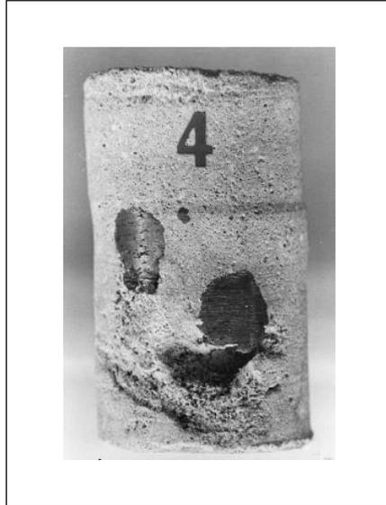
**Gambar SKh-3.7.18.4)** Kondisi Visual *Core Grade 4* Material Beton Semprot (ACI 506.2-95)
