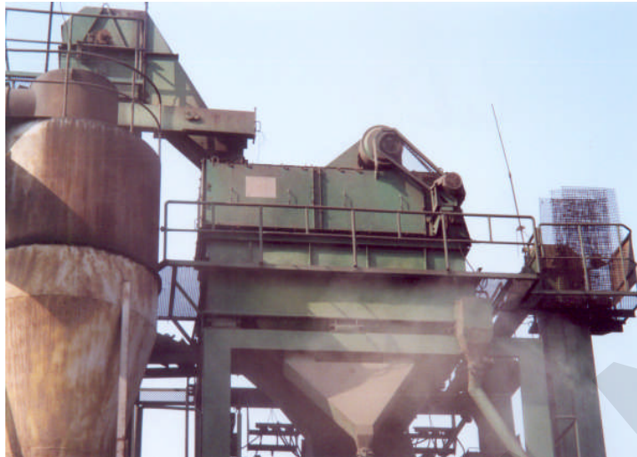
Gambar 12. Saringan Panas (Hot Screen)
