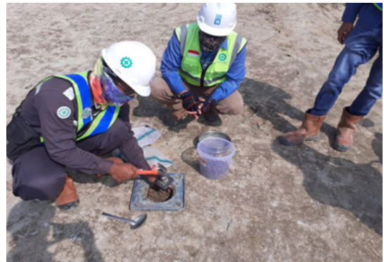
Gambar 28. Pengujian sand cone (Sumber: Work Method Statement , Satker PJT Semarang-Demak, 2023)
