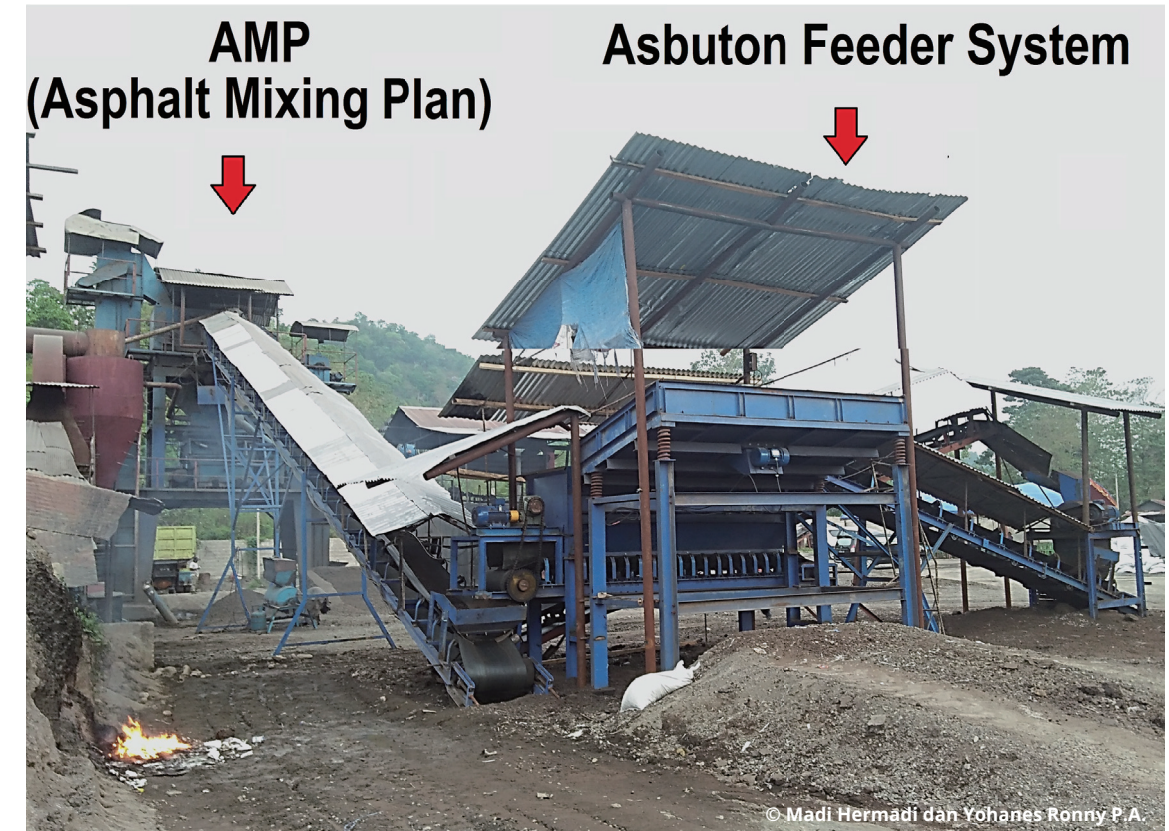
Gambar 7. Asbuton Feeder System
