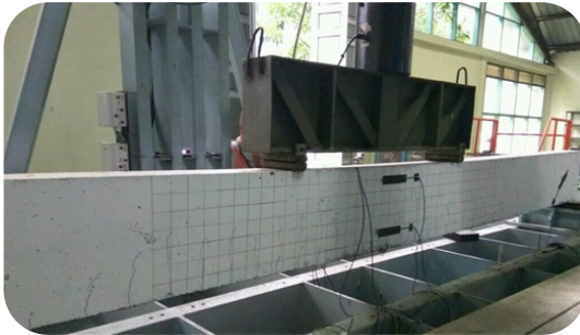
Gambar 1. Uji Coba Balok Beton TSP Sumber: Rulli Ranastra
