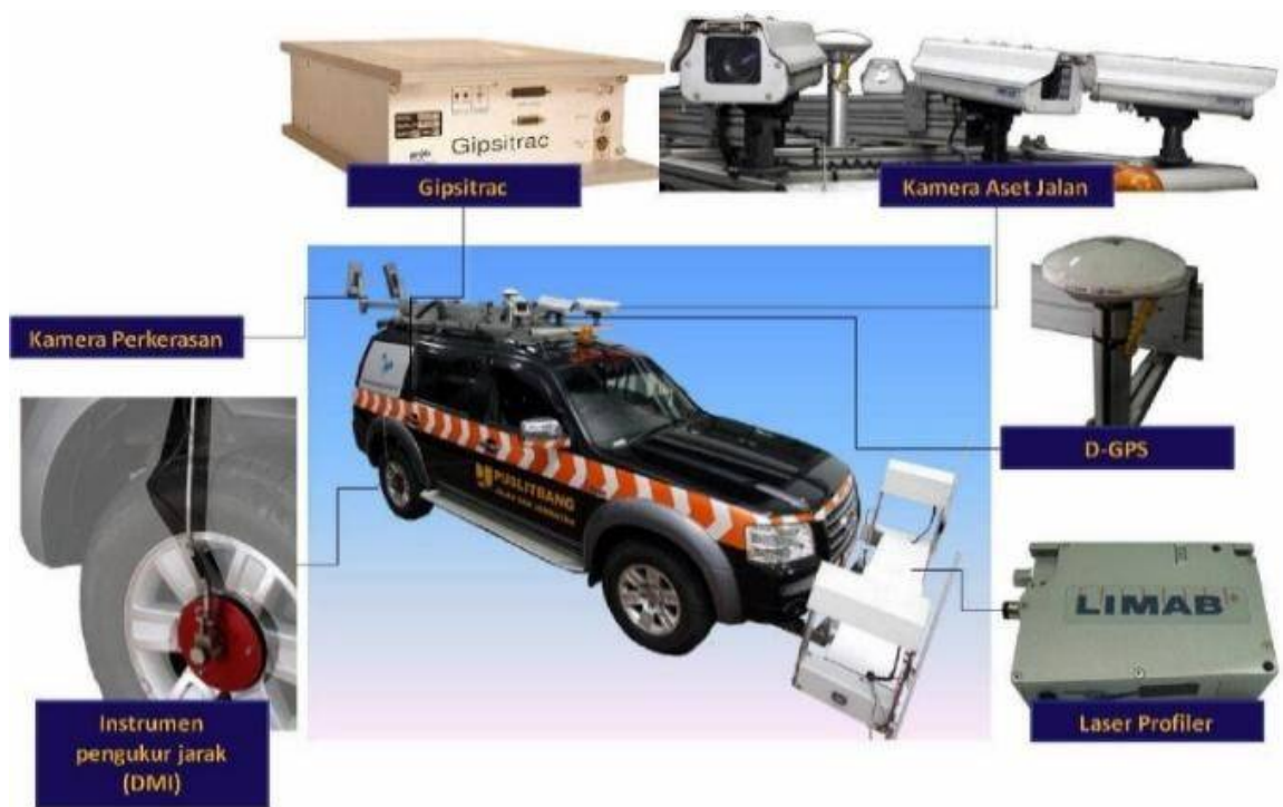
Gambar 1. Kendaraan Survey Jaringan Jalan Hawkeye 2000 series
