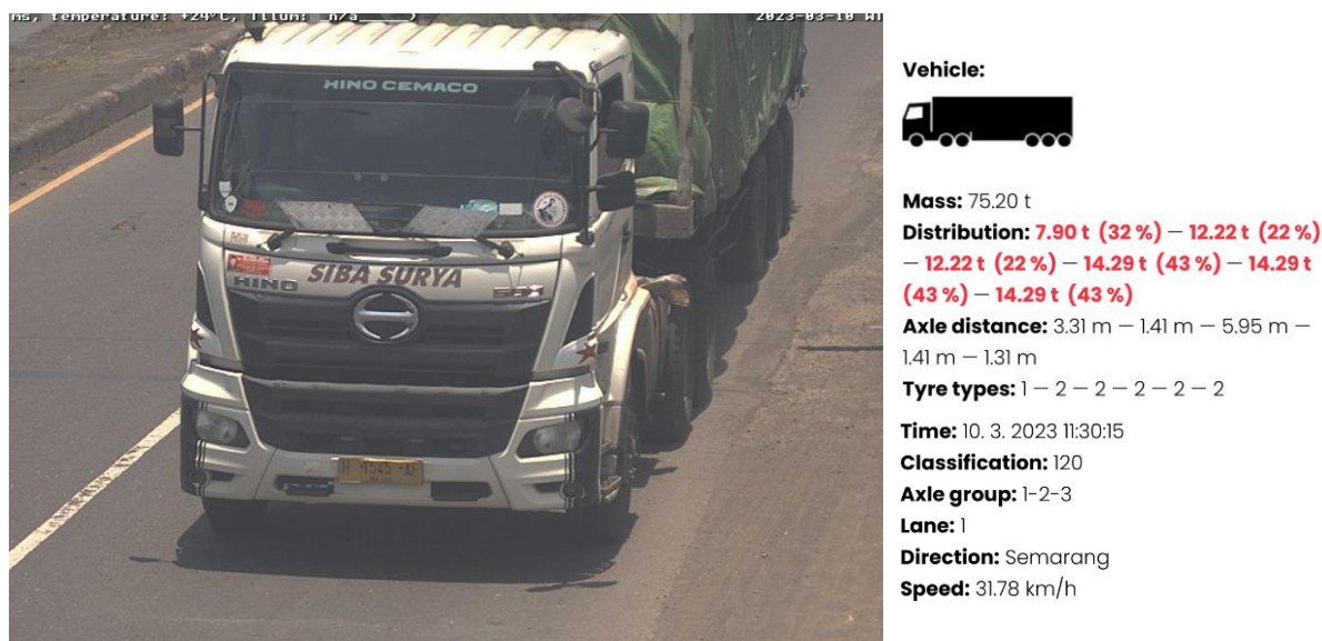
Figure 2 B-WIM measurement result example, a 6-axle vehicle with a weight of 75.20 tonf
