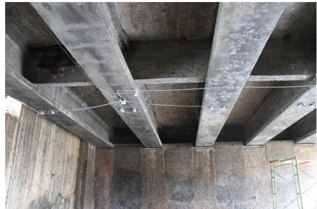
Figure 1. B-WIM Strain transducer sensors (Site ID001)
